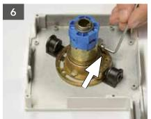
Tighten the screw on the clamping plate (screwable from both sides) with a 3 mm Allen key.
