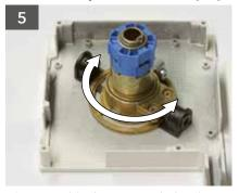
Align roughly the gear with the drive rod (45° or 90°)
