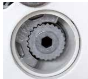
Picture 3: Tightening the screw in order to fix the gearing.
