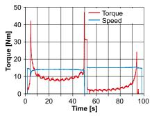
Torque diagram by extension/retraction of a folding arm awning
