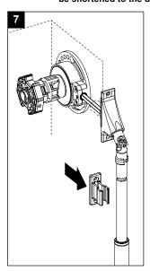
Secure the crank holder to the wall with 2 screws (not included).
