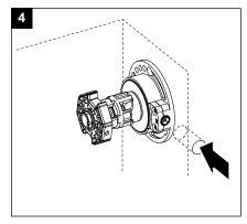
Drill a hole in the masonry at the height of the gear drive as a feed-through for the spherical bearing.
