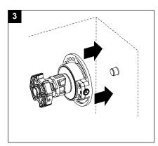
Fasten the gear to the side part of the rolling shutter box with at least 2 screws/rivets (not included in the scope of delivery).
