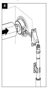
Connect the motor to the connecting cable and the mains. Slide the shaft with the installed motor onto the gear driver and set the end positions (see operating instructions of the motor).
