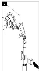
Secure the crank with the safety seal by sticking it over the holder.
