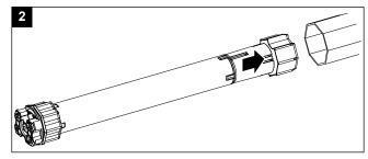
Push the motor into the 8-edge shaft.
