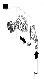
Slide the crank onto the trunnion of the spherical bearing and secure it with the supplied safety clip.
