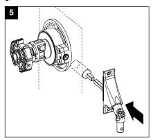
Insert the output bar of the airtight spherical bearing through the hole in the gear. Screw the spherical bearing to the wall with 2 screws (not included).
