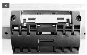
Anti-lift device is now loose on the tube ...
