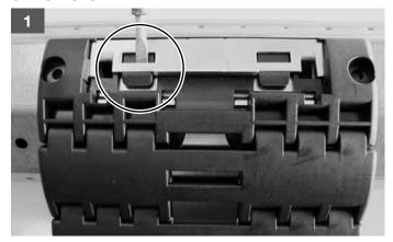
Press the plastic clip downwards with a suitable screwdriver.
