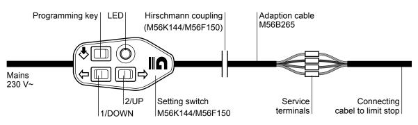
Connection with setting switch M56F151 with service terminals
