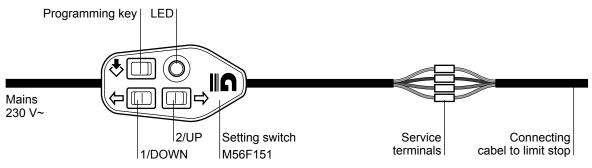
SECURITY NOTE: This setting cable is protected against damage with a fuse type T 1,6 A 250V. This fuse must be replaced by a fuse of the same type. Other types of fuse might damage the setting cable.
