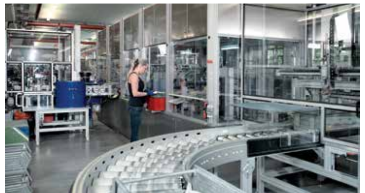
Every 3,5 seconds a crank handle is assembled from 12 components
