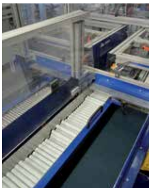
Automatic feeding process of the grips
