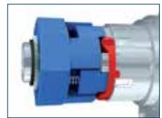
... and turn tube drive to the right until the latching elements of the overrun clutch snap into place.
