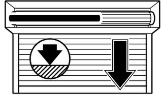
**Variant C: upper end position with stop / Lower end position freely adjustable**
