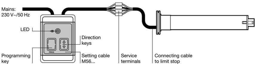
Connect setting cable to the connecting cable of the motor (see diagram on the back of the setting switch). The assignment to the direction of rotation is dependent on the installation situation of the drive. Then connect the setting switch to the 230V mains.
