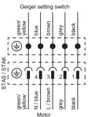
The GJ56.. E09 can be set with a standard setting switch which supplies the motor with continuous current and allows a simultaneous UP / DOWN command. In this case, instead of the programming button, the UP and DOWN buttons must be pressed simultaneously. Please connect the wires of the motor cable – respecting the colour code – with the service terminal on the GEIGER setting switch. When using different setting switches, please check the wire assignment.
