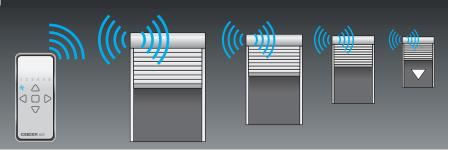
that may occur are also reported. Each motor also works as a wireless signal repeater. This means that having multiple motors guarantees a wireless coverage across the whole house, which makes it easy to overcome constructionrelated constraints such as thick concrete walls.
